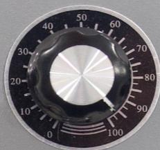
Our LED is adjustable from 10-100% with maximum power of 16 Watt/cm<sup>2</sup>. High settings allow quick curing and the best adhesion and lower LED performance can be beneficial for further production processes (CNC machining, stretching materials, etc.)
